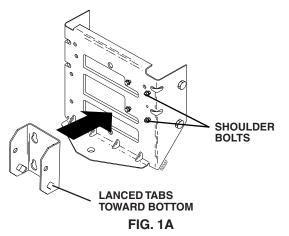
If your tractor does not have four (4) shoulder bolts installed on the drawbar, follow the instructions below.
